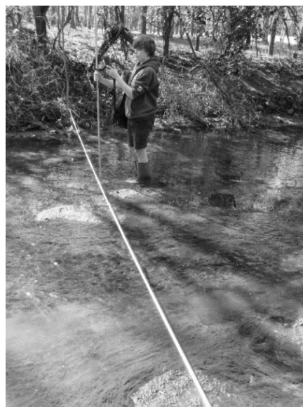
Fig 2. Setting up flow meter and tag line with measuring tape (right) (Eustace Barnes)
