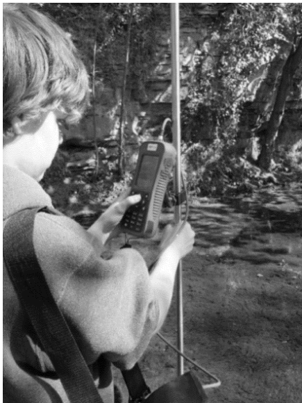
Fig 2. Setting up flow meter and tag line with measuring tape (right) (Eustace Barnes)
